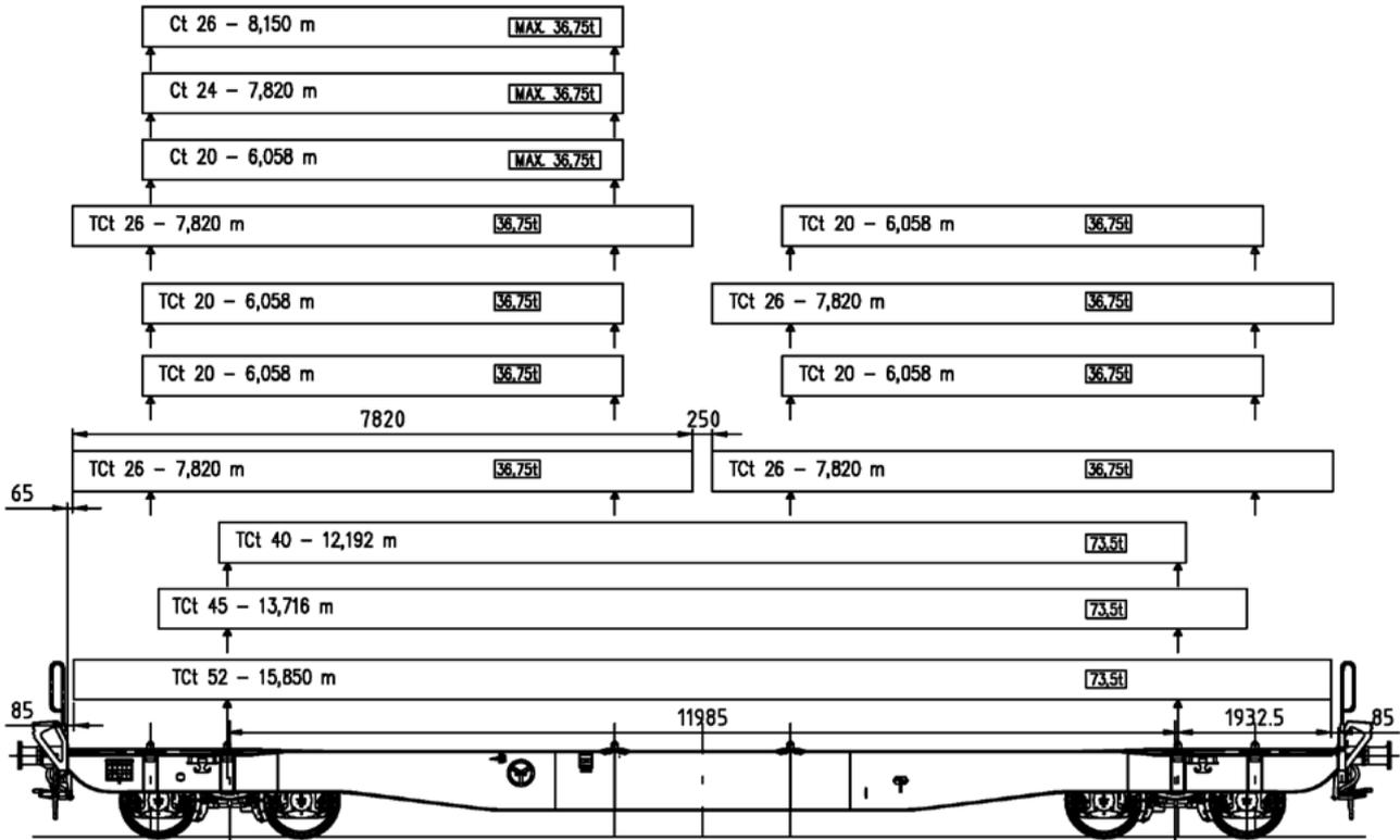
The Wascosa flex freight system® container flat wagon can be combined with the following superstructures
