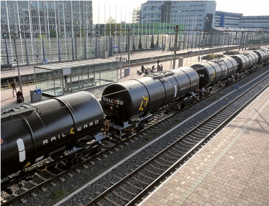
Lightweight, reliable and offering an optimal cubic capacity: The 88m3 black tank wagons, leased by Rail4ward, are Zacs from Wascosa. / Source: Rail4ward.
