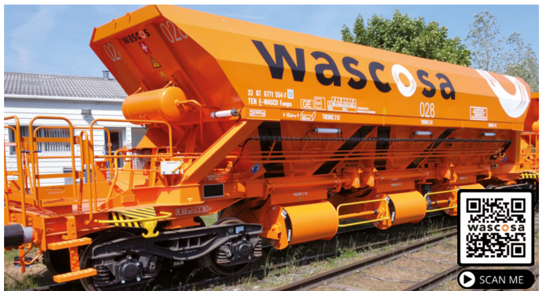
Objective achieved: The Fanps automated ballast wagon makes the work of track renewal teams much safer.
